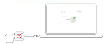
⑥ After the LauncherPlus has found the NovoPro, the main button on the LauncherPlus lights up red. Press the button to begin presenting.
