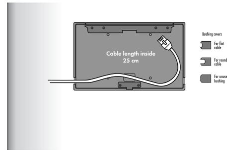
Install cable to the selected bushing and install appropriate cable cover. Cable length inside is 25 cm. Covers for flat and round cables as well as for unused bushings are delivered. Covers are fixed with adhesive tape.
