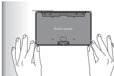
Degrease foil installed on the wall and left it completely dry. Remove protective film from the adhesive tape (installed on the rear side of the back cover) and carefully attach it on the foil installed on the wall.
