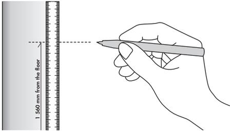
Degrease (typically glass) surface with alcohol and let it dry. Sign top of foil in height 1 560 mm from the floor. It is for recommended height 1 500 mm from floor to center of the panel.
