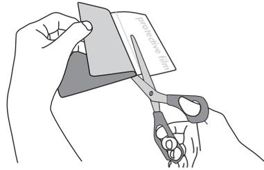
Partly remove protective film from adhesive foil and cut it.
