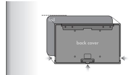
Position of back cover must be oriented as displayed above - cable bushings are left, right and below side oriented.
