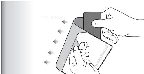
Partially remove the protective film and stick the rest of the foil using a squeegee.
