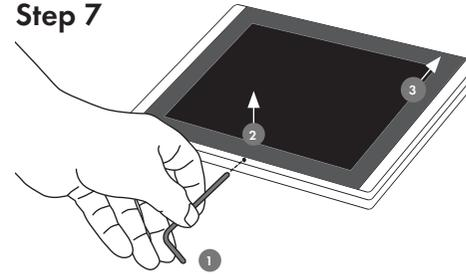
Loosen the fixing screw using delivered Allen key - ① and remove back cover of the panel - ②, ③.
