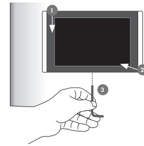
Connect Ethernet cable to the panel and put the panel on the back cover - ①, ②. Carefully tighten the fixing screw to fix panel on the back cover - ③.
