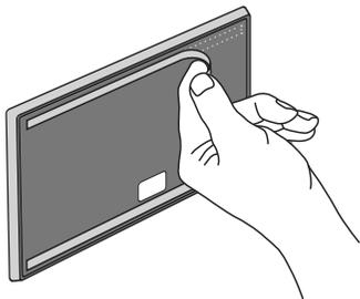
Degrease the back of the panel and attach two double-sided adhesive strips to the back of the panel. The strips should be located along the top and bottom edge of the back panel.
