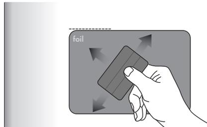
Squeegee lengthwise from the center outwards with overlapping strokes.
