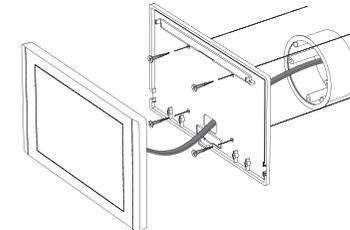
3. Install the cable so that it passes through the back cover hole. Fix back cover on the wall using appropriate screws depending on the wall material.
