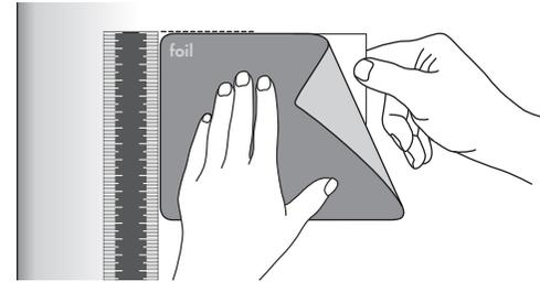
Use vertical ruler or level to adjust correct foil vertical position. Put foil on the wall with the protective film (not with adhesive part) to the ruler or level.
